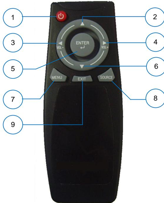
1. POWER : Turns the LCD Display On and Off
