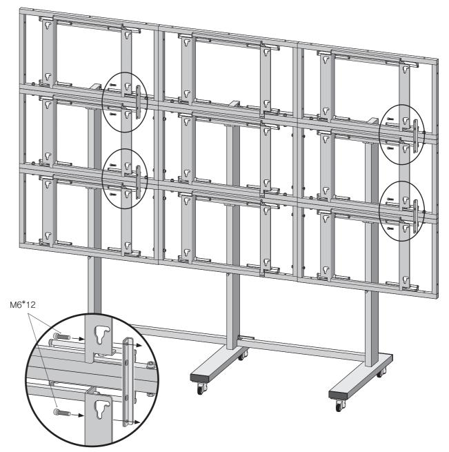
Connect the Main Frame and Y-Axis Link with M6\*12 bolts using a 5mm allen wrench.
