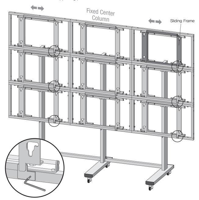
Remove the screws of the supporting plate with a 5mm allen wrench. Then, remove the plate completely from the Main Frame. - 14 -
