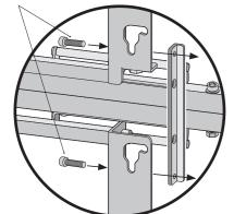
Connect the Main Frame and "Y-Axis Link" with M6\*12 bolts using a 5mm allen wrench.
