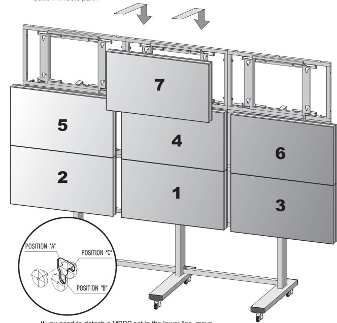
If you need to detach a MPDP set in the lower line, move the set in the upper line to position "C". Remove guide pins from the set in the lower line, move it to position "A" and detach from the main frame.
