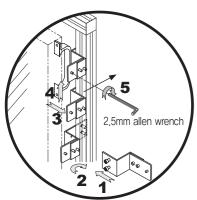
Attach the FIX BRACKET UNIT to the main frame and fix with fixing bolts next to MPDP handle. Use 2.5mm allen wrench.
