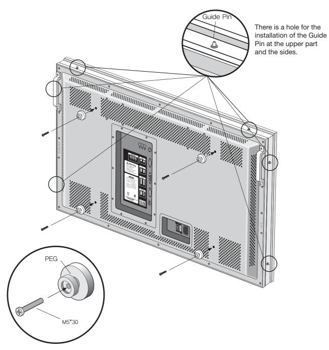
Fasten 4 PEGs in the back of MPDP with M5\*30 bolts.
